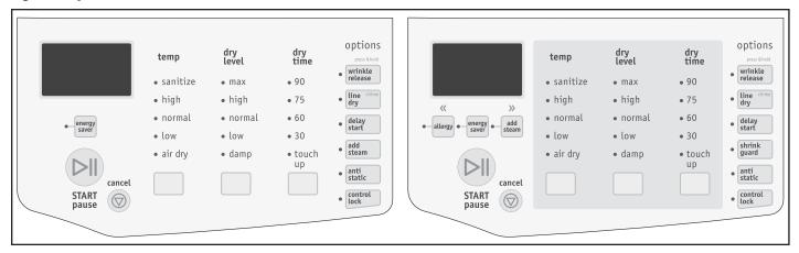
To add options, press the corresponding options buttons to illuminate the selections desired. To delete options, press the options buttons again and the indicator lights will turn off. Some options require a "Press & Hold" effort to activate or deactivate the secondary function.
