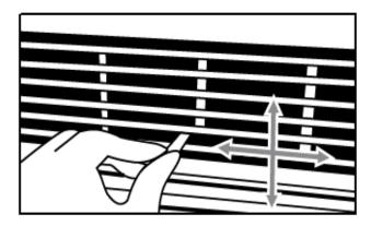
The 4-way air directional louvers allow you to direct the air flow Up, Down, Left, and Right throughout the room as needed. To adjust the air directional louvers side to side use the center handles as you move side to side. To pivot the louvers, press with your fingers until the desired airflow direction is obtained.
