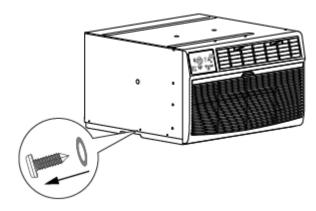
2. The ground wire will be attached to the air conditioner cabinet using the screw you just removed along with a Toothed Washer.
