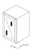
It is important for the wine cooler to be leveled in order to work properly. It can be raised or lowered by rotating the plastic sheaths around each of the feet on the bottom of the machine. If you find that the surface is not level, rotate the feet until the wine cooler becomes level. You may need to make several adjustments to level it. We recommend using a carpenter's level to check the machine.
