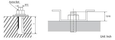
Figure 15: LMU183HV and LMU243HV Outdoor Units.
