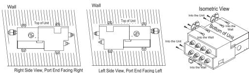
Figure 23: Unacceptable Branch Distribution Unit Wall Mount Orientations.
