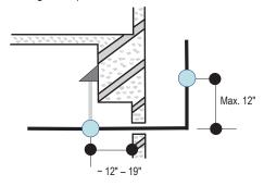
Figure 32: Pipe Support at Indoor Unit.
