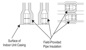
Figure 67: Insulating the Shut Off / Isolation Ball Valve (If Present).
