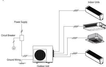
Figure 82: Typical Multi F MAX System General Power / Communications System Schematic.
