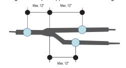
Figure 34: Pipe Support at Header Fitting.
