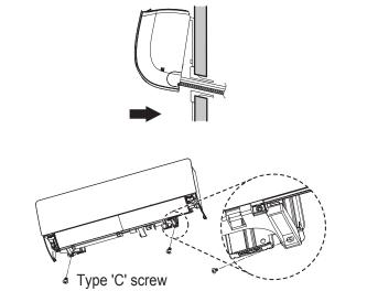
6. Finish the installation by completely securing the indoor unit to the installation plate using the factory-supplied screws (screw placement will vary depending on indoor unit model).
