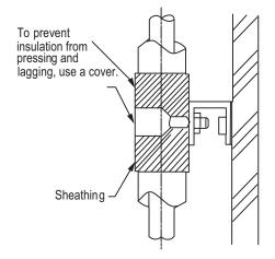
Figure 39: O-Ring Band Support with an Insulated Pipe.
