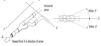
Figure 61: Y-branch Installation Alignment Specification.
