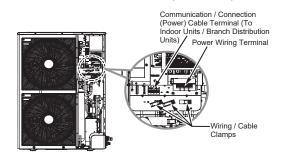
Figure 90: Connecting the Power Wiring / Communica-
