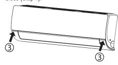
Figure 96: Checking that All Attachment Locations Are Secure (Step 5).
