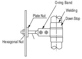
Figure 41: Two-Point Down-Stop Support.
