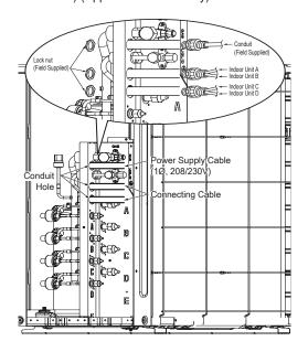
Figure 89: Connecting the Power Wiring / Communications Cables to the Outdoor Unit (LMU481-541HV).
