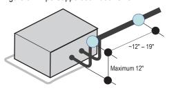
Figure 33: Pipe Support at Y-branch Fitting.
