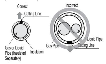
Figure 69: Piping with Insulation Material.
