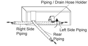
Figure 28: Bending Piping at Rear of Indoor Unit.
