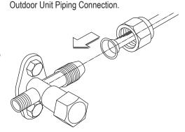
Figure 46: Close Up of the Field Piping to the
