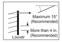
Figure 9: Using "S" Type Louvers.
