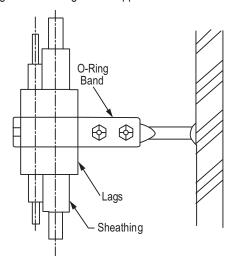
Figure 40: One-Point Down-Stop Support (>441 lbs.).
