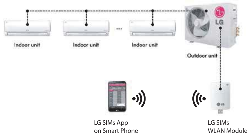
Figure 106: SIMS WLAN Module to Typical DFS System
