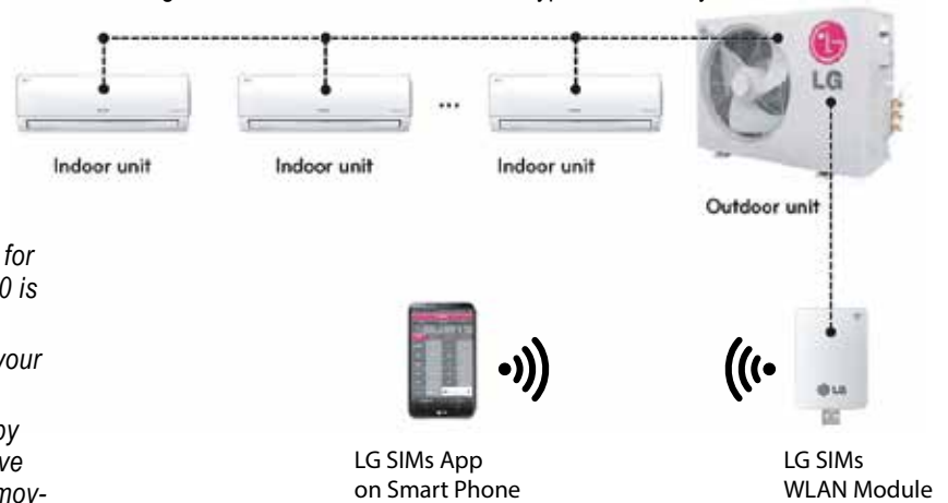
Figure 64: SIMS WLAN Module to a Typical Multi F System.
