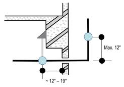
Figure 28: Pipe Support at Y-branch Fitting.
