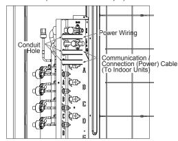
Figure 89: Multi F MAX with LGRED Outdoor Unit Wiring Connections Close Up View (LMU300HHV Example).
