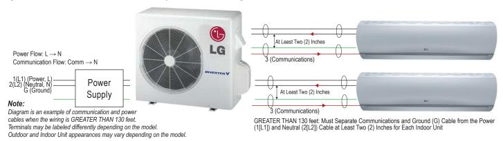
Figure 83: Schematic of a Multi F MAX with LGRED System When the Wiring is GREATER THAN 130 Feet.
