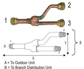
Figure 20: Y-branch Horizontal Installation Alignment.
