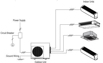
Figure 81: Typical Multi F MAX with LGRED System General Power / Communications System Schematic When Wiring is Less Than 130
