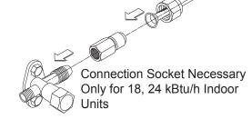
Figure 44: Connection Socket Diagram, External View.
