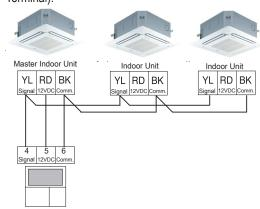
Figure 99: Example of Indoor Unit Group to Zone Controller Connections (CN-REMO).
