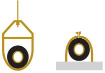
Ise a 4" + long sheet curved sheet metal saddles between hanger bracket and insulation to promote linear expansion/contraction.
