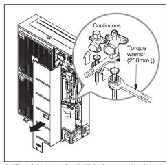
\* When tighten the pipe, hold the haxagonal body.
