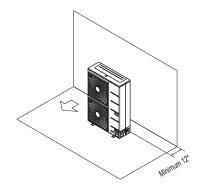
Obstacles on the suction side and on both left and right sides.
