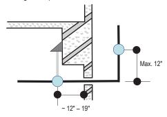
Figure 28: Pipe Support at Indoor Unit.
