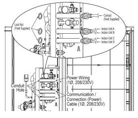
Figure 90: Multi F MAX with LGRED Outdoor Unit Wiring Connections (LMU360HHV Example).
