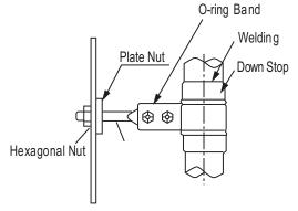
Figure 37: Two-Point Down-Stop Support.
