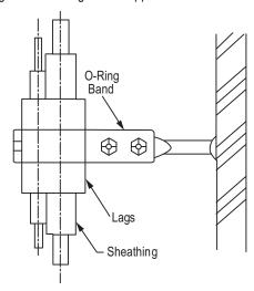
Figure 36: One-Point Down-Stop Support (>441 lbs.).
