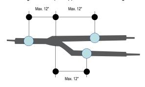
Figure 27: Pipe Support at Indoor Unit.
