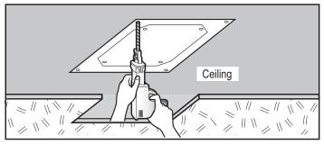
Figure 8: Ceiling Opening Dimensions and Bolt Locations.
