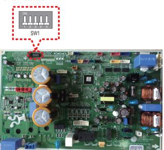
Figure 114: Multi F MAX with LGRED (LMU360-420HHV) Outdoor Unit DIP Switch Locations.
