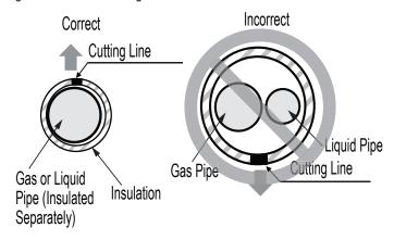
Figure 67: Piping with Insulation Material.
