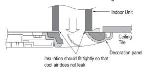
Figure 57: Installing the Decoration Grille Kit.
