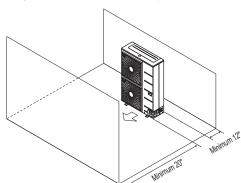
Where there are obstacles on both suction and discharge sides (discharge side obstacle is lower than the outdoor unit).
