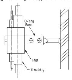
Figure 34: One-Point Down-Stop Support (>441 lbs.).
