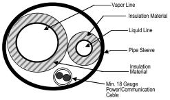
Figure 38: Underground Refrigerant Piping.
