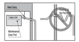
Figure 15: Flexible Drain Hose Connection.
