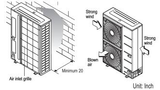
Ensure that the space at the back of the outdoor unit is a minimum of 12 inches, and include a minimum of 24 inches at the right side of the unit for service.
