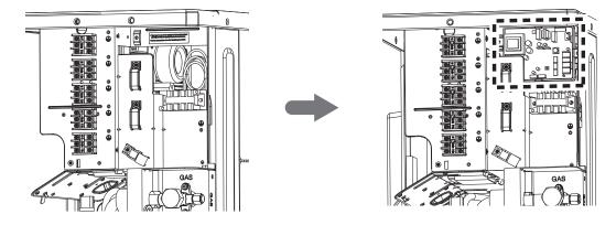
Figure 94: PI-485 Board (Appearance will differ depending on model).
