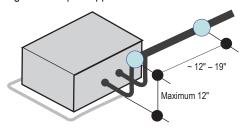
Figure 29: Pipe Support at Y-branch Fitting.
