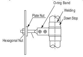
Figure 35: Two-Point Down-Stop Support.
