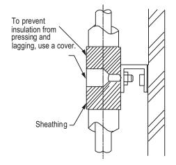
Figure 35: O-Ring Band Support with an Insulated Pipe.
