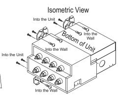
Figure 18: Unacceptable Branch Distribution Unit Orientation.
