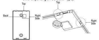
Figure 71: Installing / Removing
