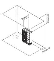
ce side. Obstacles above, on the air intake side, and on both left and right sides
