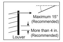
Figure 7: Using "S" Type Louvers.
