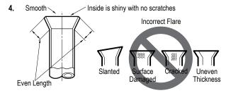
Flared Connection Dimensions / Tightening Torque.
