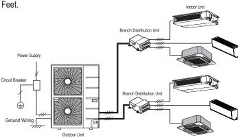
Figure 82: Schematic of a Multi F with LGRED System When the Wiring is GREATER THAN 130 Feet.
