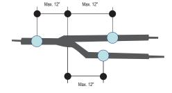
Figure 30: Pipe Support at Header Fitting.
