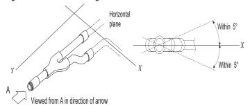
Figure 56: Y-Branch Port Identifier Diagram.
