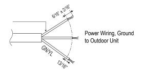
Power Wiring, Ground, Communication Cable From Outdoor Unit To Indoor Unit or from the Outdoor Unit to the Branch Distribution Unit
