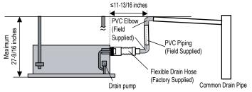
Figure 13: Drain Slope.
