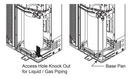
Figure 48: Filling Access Holes in the Outdoor Units.
