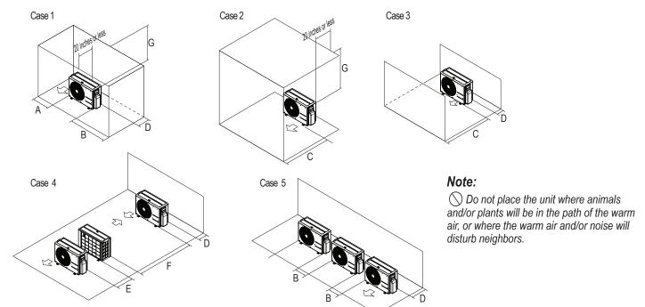
Table 8: Multi F with LGRED 18,000, 24,000, and 30,000 Outdoor Unit Service Access and Allowable Clearances Diagram Legend
