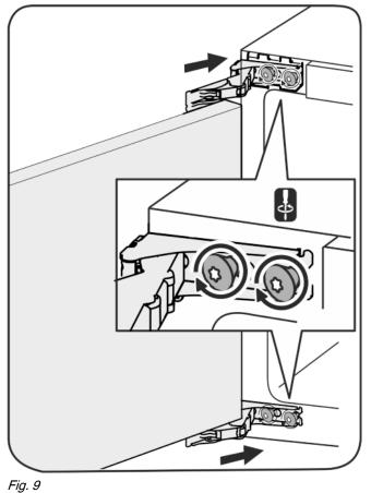
➤ Fitting the door again: Reattach the door to the hinges and tighten the screws.
