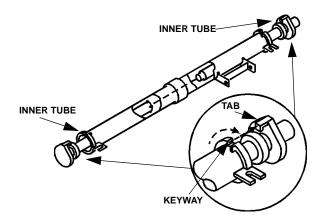
**Water Distribution Tube Disassembly**
