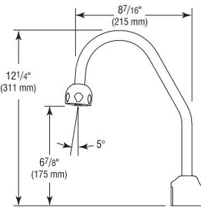
† The wide Spray Head is recommended for use on scrub or deep wash-up sinks only. For lavatories and small basins, use the Laminar Flow Spray Head.
