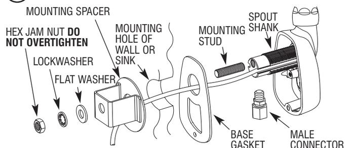
**Note:** Sloan Valve Company does **NOT** supply hardware necessary for mounting the Faucet on surfaces thicker than 1" (25 mm).
