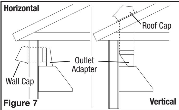
**NOTE:** For models using the B300, B500, or B600 blowers, a minimum of 6" diameter outlet adapter & ducting is required to achieve the proper air flow. The B900 requires a minimum 8" diameter adapter and ducting, while the B1125 requires a minimum 10" diameter adapter and ducting.
