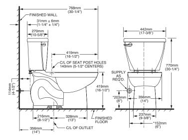
NOTES: THIS TOILET IS DESIGNED TO ROUGH-IN AT A MINIMUM DIMENSION OF 356MM (14") FROM FINISHED WALL TO C/L OF OUTLET. SUPPLY NOT INCLUDED WITH FIXTURE AND MUST BE ORDERED SEPARATELY.
