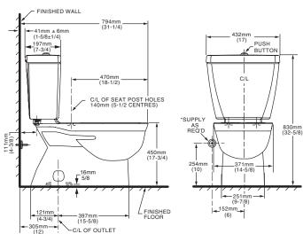
THIS TOILET IS DESIGNED TO ROUGH-IN AT A MINIMUM DIMENSION OF 305MM (12") FROM FINISHED WALL TO C/L OF OUTLET. SUPPLY NOT INCLUDED WITH FIXTURE AND MUST BE ORDERED SEPARATELY.
