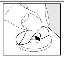
Remove the paper backing from one side of the washer.
