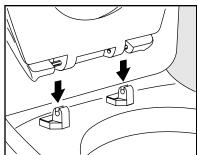
After cleaning, replace seat into hinge posts. Push down on one side then the other.
