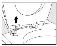
First raise the seat and cover. Pull up one side then the other and remove seat.
