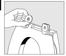
Attach washer to bottom of hinge. Remove paper backing.
