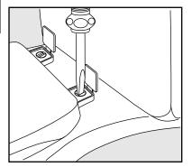
Use a screwdriver to tighten bolt.
