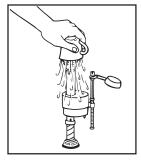
While holding a container over the uncapped VALVE to prevent splashing, turn water supply on and off a few times. Leave water supply off.
