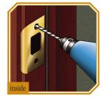
8 For Latch Strikeplate: Using latch stikeplate as a template, drill two 1/8" pilot holes for the  $\#8 \times \frac{3}{4}$ " screws.
