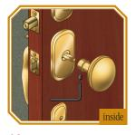
13 Slide knob onto spindle and tighten set screw with Allen wrench. Knob/lever is secured when set screw enters V groove in spindle.
