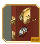
Place inside turnpiece over mounting plate. Insert tailpiece into inside turnpiece. Attach inside turnpiece to mounting plate with two #8-32 x 3/4" oval head screws. Make certain turn knob rotates smoothly in both directions.
