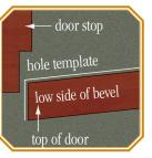
2 (Aerial View) To ensure proper alignment, only use hole template on side facing Helpful Hint: Some doors have a beveled edge with bevel facing doorstop.
