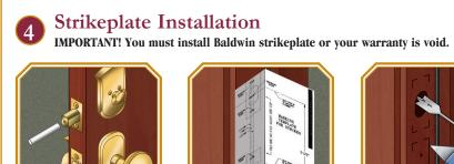
2 On doorframe, align strike hole template with center point. Mark holes for center of latch bolt and outer corners of both strikes with pencil.
