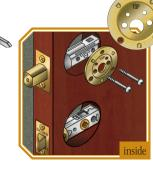
**6** Place turnpiece mounting plate on inside of door. Attach to cylinder using two #10-32 x 1<sup>7</sup>/<sub>8</sub>" pan head screws. Tighten screws. Important: Note orientation of mounting plate.
