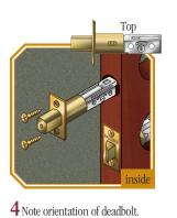
Insert deadbolt. Drill ½" pilot holes. Secure with #8 x 3/4" combinations screws so latch is flush with door.
