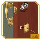
8 Attach handle by inserting the #10-32 x 2<sup>3</sup>/<sub>4</sub>" oval head screw on inside of door through screw base and the lower hole (E). Leave screw loose for adjustment. Note: Go to door preparation if you do not have a lower hole (E).
