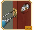
**3** Insert latch with angled side of bolt facing outside. Drill 1/8" pilot holes. Secure with #8 x "' combination screws so latch is flush with door. Repeat for deadbolt.
