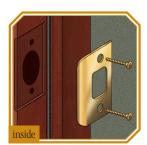
9 For Latch Strikeplate Insert dustbox into hole, add strikeplate, and secure by inserting #8 x <sup>3</sup>/<sub>4</sub>" wood screws into pilot holes.
