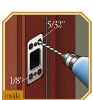
**5** For Deadbolt Strikeplate: Using reinforcing strikeplate as a template, drill two <sup>5</sup>/<sub>32</sub>" pilot holes for 3" long screws (outside holes) and two 1/8" pilot holes for #8 x <sup>3</sup>/<sub>4</sub>" screws (inside holes).
