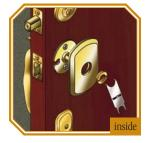
**14** Position rosette onto inside adapter. Using rose retainer wrench, thread the rose retainer onto the threaded portion of the adapter.
