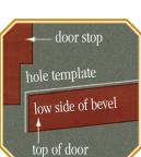
2 (Aerial View) To ensure proper alignment, only use hole template on side facing doorstop Helpful Hint: Some doors have a beveled edge with bevel facing doorstop.
