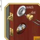
**7** Keeping tailpiece vertical and curved toward right side of hole, insert inside cylinder through inside cylinder collar base, aligning slot on top of inside cylinder with notch on insid cylinder collar base, into deadbolt. Secure with two #10-32 x  $2\frac{1}{4}$ " flat head screws.
