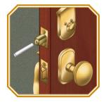
If weather stripping is not installed, you must install weather stripping prior to strikeplate installation. Mark center of deadbolt with chalk, grease pencil, or lipstick. Shut door and lock deadbolt to mark center point on doorframe.
