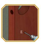
**7** Very carefully drill (C, D) holes **8** Very carefully drill (E)  $\frac{1}{16}$ hole into door exactly at pencil mark.
