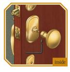
**15** Slide knob onto spindle and tighten set screw with Allen wrench. Knob/lever is secured when set screw enters V groove in spindle.
