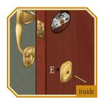
11 Attach outside handleset trim by inserting the #10-32 x 2<sup>3</sup>/<sub>4</sub>" oval head screw on inside of door through screw base and the lower hole (E). Leave screw loose for adjustmen Note: Go to door preparation if you do not have a lower hole (E).
