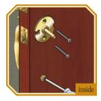
**13** Align spindle, latch, and outside handle. Insert the inside adapter onto the posts of the outside handleset trim. Secure outside handleset trim so spindle with two  $\#10-32 \ge 1\frac{1}{4}$ " flat head screws. Tighten all three screw including screw for bottom of handle.
