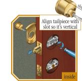
**O**Extend deadbolt with flat head screwdriver. Keeping tailpiece vertical and toward the right side of hole, insert outside cylinder through itside cylinder collar, the into deadbolt. Hold in place. Note: Do not insert key.
