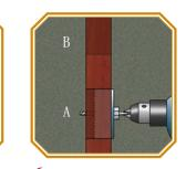
Complete drilling holes (A, B) from opposite side of door.
