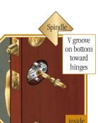
12 From inside of door, insert short end of spindle through the latch with the V groove angled down and toward hinges. Position slides into square hole in thumbpiece cartridge. Note: Make certain spindle is completely inserted up to stops.
