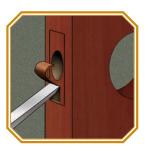
**10** Chisel faceplate cavity Helpful Hint: Chisel toward inside edge of score lines, removing only a small bit to avoid wood damage.
