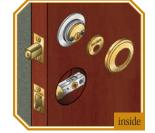
9Align inside cylinder cap over inside cylinder. Screw on inside cylinder collar.
