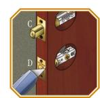
**9** Insert latch into hole (D). Use utility knife to score chisel guides into door edge. Make sure score guides are parallel to door. Repeat for deadbolt hole (C).
