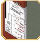
**5** Fold hole template along door edge with center of bottom hole (A), the  $2\frac{1}{8}$ " dia. hole, 38" from floor. Tape template to door.
