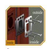
**6** For Deadbolt Strikeplate: Insert dustbox into hole, add reinforcing strike, and secure with 3" reinforcing screws (outside holes) and #8 x <sup>3</sup>/<sub>4</sub>" combination screws (inside holes). Helpful Hint: When installing wood screws it is recommended to put beeswax or soap on screw threads to improve installation.
