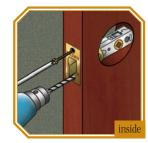
**5** Insert latch with angled side of bolt facing outside. Drill 1/8" pilot holes. Secure with #8 x 3/4" combination screws so latch is flush with door. Repeat for
