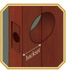
Determine your backset, which is the distance from the edge of door to center of hole. Your lockset is shipped with a 2<sup>3</sup>/<sub>8</sub>" backset (most ommon). Adjust for a 2¾ backset door only.
