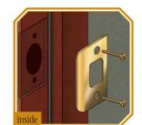
**9** For Latch Strikeplate Insert dustbox into hole, add strikeplate, and secure by inserting #8 x ¾" wood screws into pilot holes.
