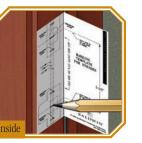
**2** On doorframe, align strike hole template with center point. Mark holes for center of latch bolt and outer corners of both strikes with pencil.
