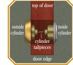
**8** (Aerial view) Align tailpiece with slot. Keep tailpiece vertical and curved toward right side of hole. Note: Cylinder tailpieces must meet each other as shown.
