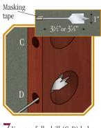
into door edge exactly at pencil  $3\frac{1}{2}$ " deep for a  $2\frac{3}{8}$ " backset  $3\frac{7}{8}$ " deep for a  $2\frac{3}{4}$ " backset Helpful Hint: Mark edge depth of drilling with masking tape.
