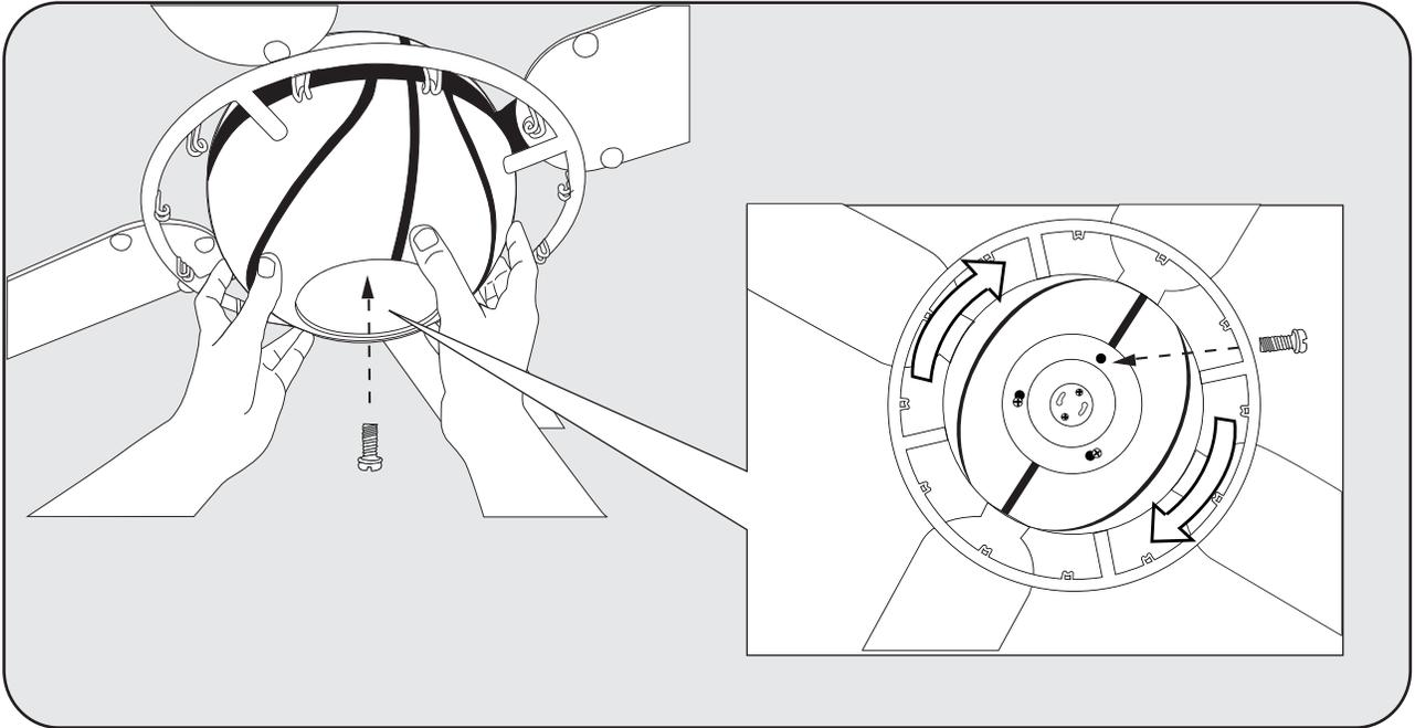
Seat Light Kit (5) into position and lock into place by twisting 1/4 turn. From light kit hole screw set screw into place firmly.
