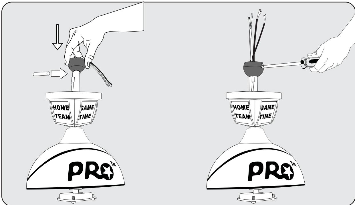
Replace hanging ball, insert hanging pin through downrod and tighten ball screw through hanging ball into downrod.
