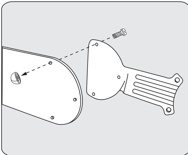
Assemble Blade (11) to Blade Arms (8) by inserting screw (S4) and securing with Blade Medallion (10).
