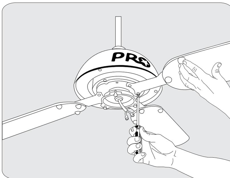
Support and attach Blade Assembly to Motor with Motor Screws (S2)
