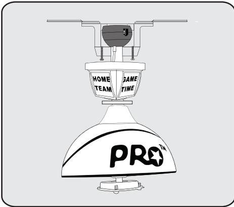
Attach Canopy Night Light (3) to the mounting bracket by placing canopy screws into keyed hole slots.
