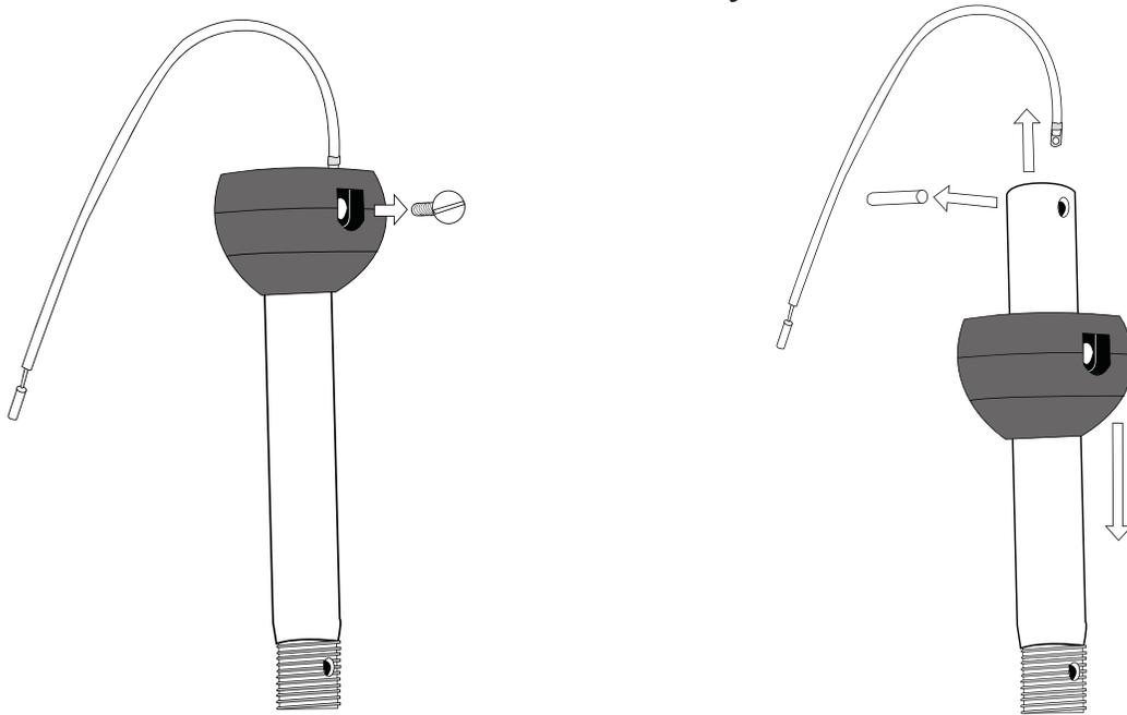
Locate downrod assembly (2). Loosen ball screw on black hanging ball to free lock pin. Black hanging ball will slide down. Remove ground screw and green ground wire. Remove hanging ball from downrod and save all parts.
