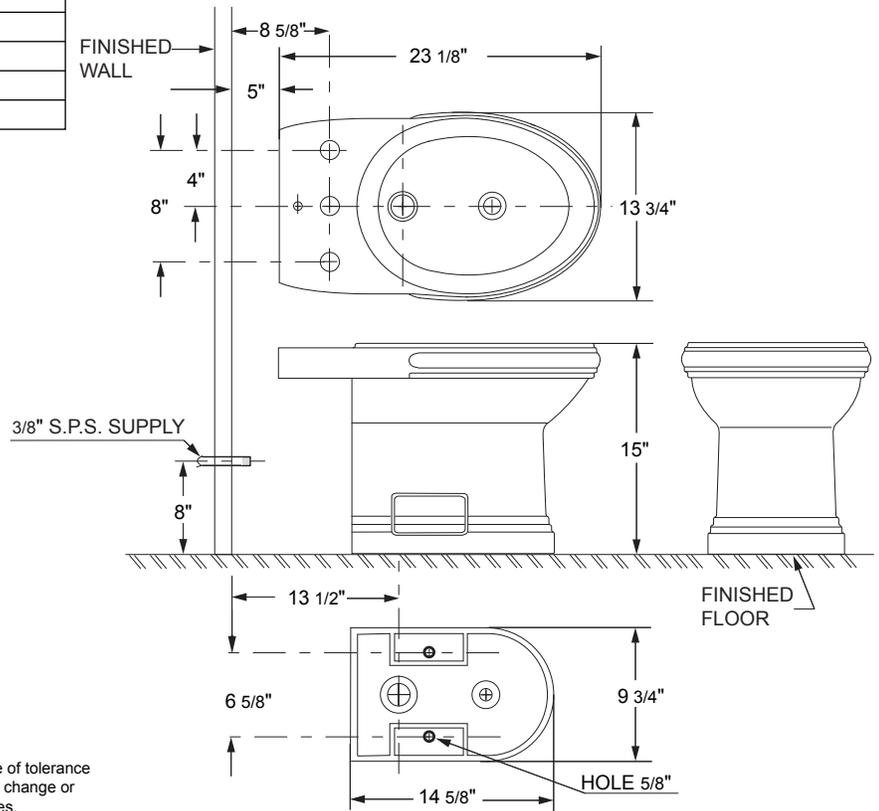
IMPORTANT: Dimensions of fixtures are nominal and may vary within the range of tolerance established by ASME Standard A112.19.2. These measurements are subject to change or cancellation. No responsibility is assumed for use of superseded or voided pages.
