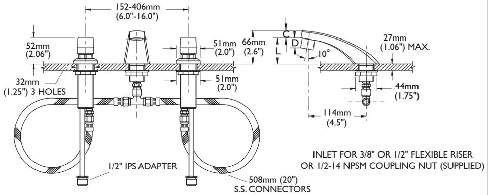
INLET FOR 3/8" OR 1/2" FLEXIBLE RISER OR 1/2-14 NPSM COUPLING NUT (SUPPLIED)
