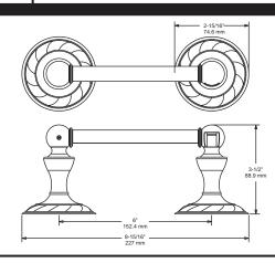
MATERIALS: Posts and Bar - Zinc Die Cast Wall Plate - Steel, Nickel Plated
