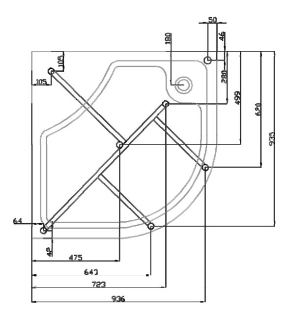
Fig 1 Legs and frame position (top view)
