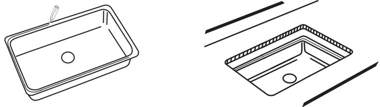
**3** From the underside, lightly tighten the fasteners with a screwdriver until the sink is snug against the countertop.
