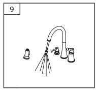
FAUCET OPERATION AND INSPECTION Turn on hot and cold water supplies. Pull the hose assembly out of the spout and remove the spray head. Be sure to hold the end of the hose down into the sink and turn faucet handle to the mixed position. Flush water lines for one minute. Check for leaks. Re-tighten if necessary, but do not overtighten. Reinstall the spray head tight.
