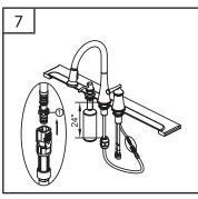
HOSE INSTALLATION Align block (1) onto hose. Install quick connect onto spray hose. Push quick connect firmly onto outlet hose tab. Install weights onto spray hose. Locate the weights 24" from the underside of the sink deck.
