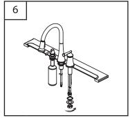
Insert handle assembly through mounting holes in sink. From under sink, install rubber washer, metal washer and nut onto the mounting shank.
