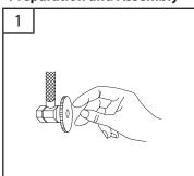
Locate water supply inlet and shut off water supply valve. These are usually found under the sink or near the water heater. Remove old faucet. Clean and dry sink surface area where new faucet will be mounted.
