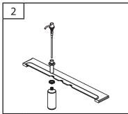
FOR MODELS WITH SOAP DISPENSER Remove the bottle. Separate head from body assembly. Make sure flange is properly seated in the base of the body assembly. Insert body assembly through selected hole in sink. Secure body assembly to sink with nut. From under the sink, screw the bottle onto the body assembly shank, then attach head assembly.
