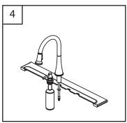
MOUNT FAUCET TO DECK Insert faucet through mounting holes in sink. Your faucet is designed for a hole diameter of 1-3/8" ± 1/4" (35mm ± 6mm) and a deck thickness of up to 2-1/2" (64mm).
