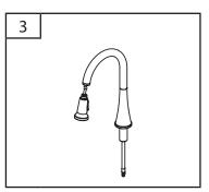
ATTACH SPOUT TO VALVE Feed hose assembly through spout and hub. Attach sprayer to end of hose to keep hose in place. Rotate spout assembly to ensure smooth operation
