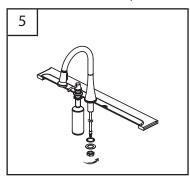
From under sink, install rubber washer, metal washer and nut onto the mounting shank.
