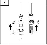
Make connections to water lines. Use 1/2" IPS faucet connections (1) or use supplied coupling nuts (3) with 3/8" OD ball-nose riser (2). Do not overtighten.
