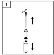
Remove the bottle. Separate soap dispenser head from flange body assembly.
