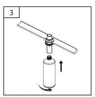
Screw bottle clockwise onto body assembly shank.
