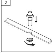
Insert body assembly through selected hole in sink. Secure body to sink by screwing the mounting nut from the underside of the sink clockwise. Hand tighten only.
