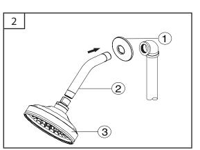
Insert the long end of the shower arm through the flange (1) then apply pipe tape or pipe thread compound to both ends of shower arm (2). Screw the long end of the shower arm into the pipe elbow inside the wall. Slide the flange (1) tight against the finished wall surface. Thread the shower head (3) onto the shower arm (2).
