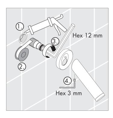
The 12 mm allen wrench shown is not included. 12 mm allen wrenches are available at hardware and auto parts stores.
