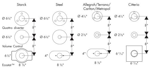
The positions of the valves can be adjusted for the tile pattern. However, care must be taken to leave enough space for the trim plates.
