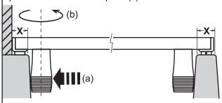
**BUMPER INSTALL.** If required, install the extra bumpers directly to the wood. Carefully drill a pilot hole for the (supplied) #6 pan head wood screws. Ensure the bumpers are aligned with factory-installed bumpers as shown in Bottom View.
