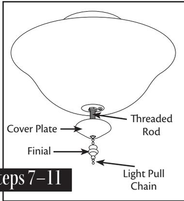
7. Install two 60-watt maximum Type B-10 (candelabra) bulbs into the lamp sockets.
