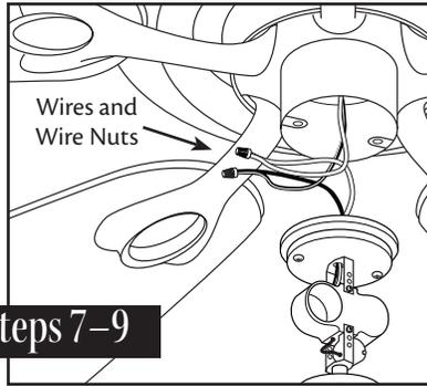
7. Remove the wire nuts from the two wires in the switch housing labeled “Connect Light Here” or “For Light Use.” One wire is white and the other wire is black/white striped.
