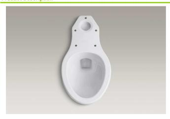
The elongated bowl toilet shall be made of vitreous china. Toilet shall be 30-1/8" (765 mm) in length, 21-1/4" (540 mm) in width, and 31-1/4" (794 mm) in height with an 11-1/2" (292 mm) by 9-1/2" (241 mm) water area. Toilet shall be 12" (305 mm) rough-in. Toilet shall feature 2-1/4" (57 mm) glazed trapway. Toilet shall be less seat and supply.
