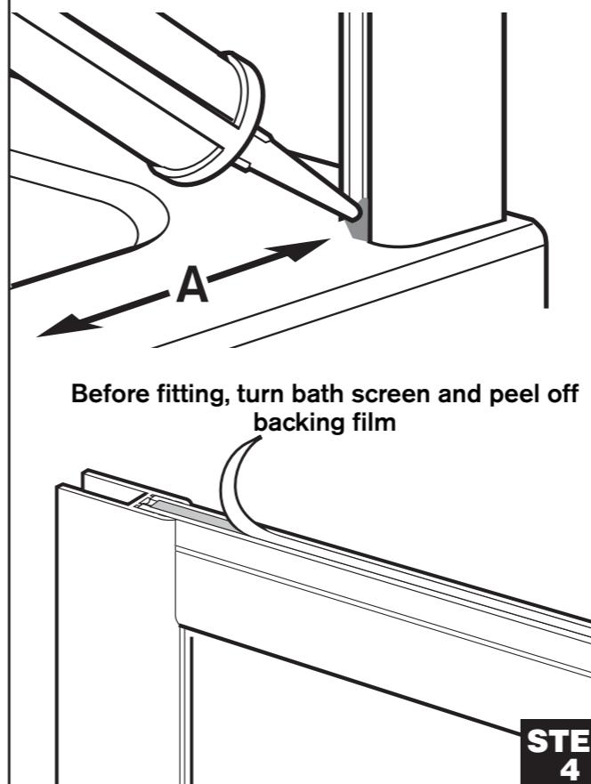
Fold the screen. Have one person carefully lift the screen and place it in the wall channel. At the same time a 2nd person needs to guide the bottom edge so that it is parallel to the front edge of the bath as it is being stuck down.
