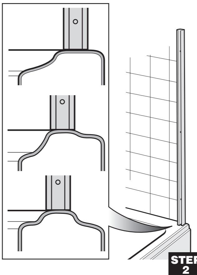
Clean & dry top of bath 'A'. Place a blob of sealant in the wall channel
