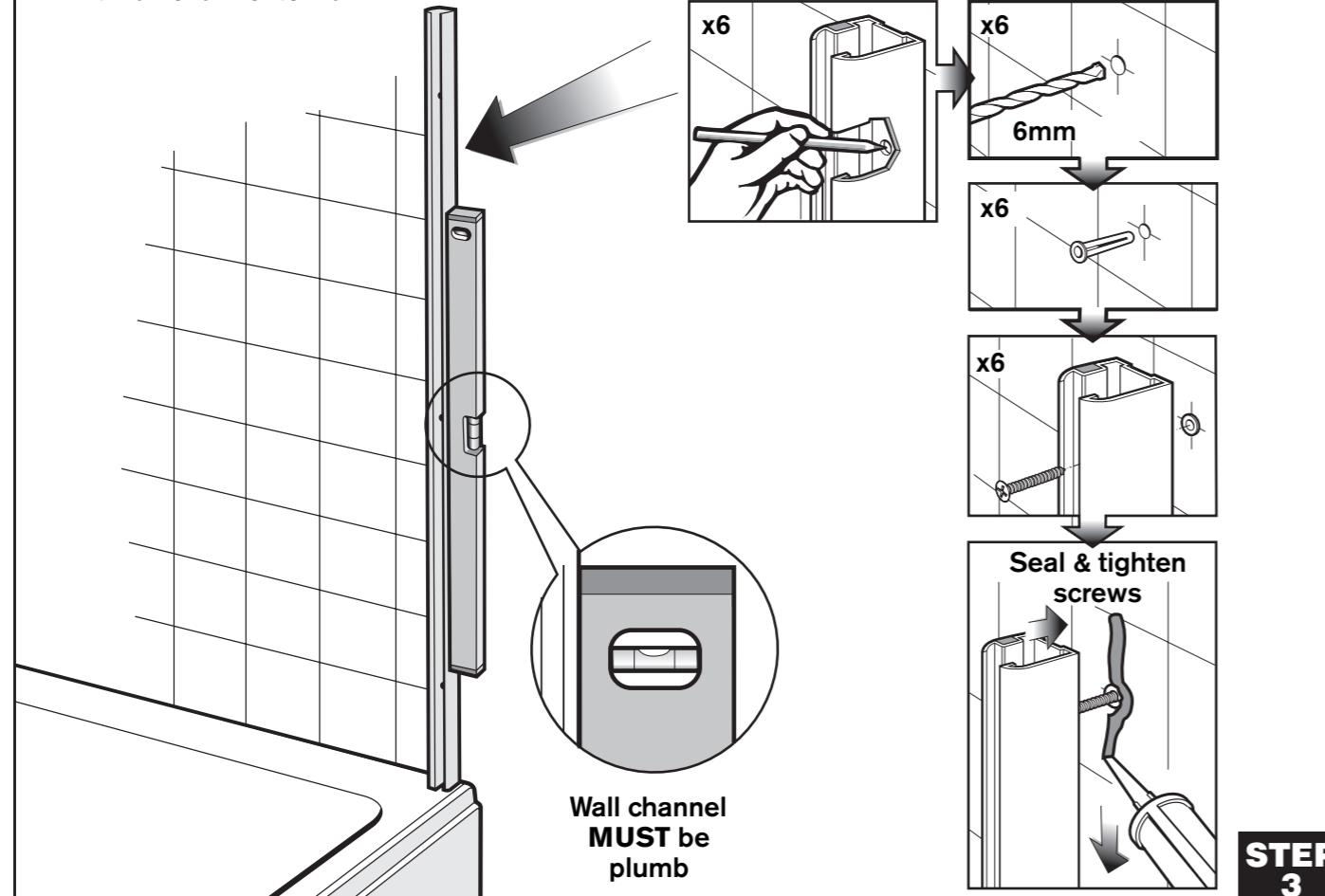
Pull back seal, drill holes through wall channel and secure screen with screws
