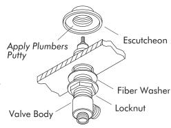
Align the valve body outlets with Supply Inlet Tube the rigid supply inlets.
