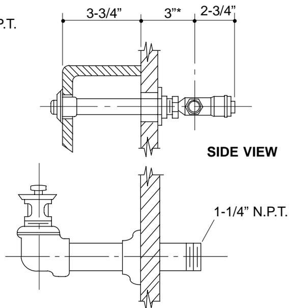
\* SUPPLY FITTING REQUIRED FURNISHED FOR WALL NOT TO EXCEED 1" THICK. FOR THICKER WALL ADD 1" TO SUPPLY MEASUREMENT (3") FOR EVERY INCH OR FRACTION THEREOF.
