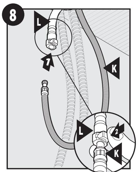
**NOTE: To ensure proper operation:** Locate white indicator mark on hose **K1**. Install weight **G** on side of hose with white indicator mark. Install hose weight just above the start of loop curvature in hose.
