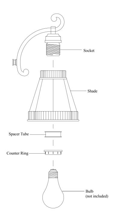
This product can be installed onto a wall either with a glass shade facing up or down.
