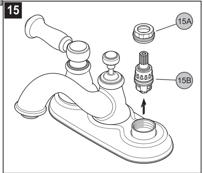
**15 VALVE CARTRIDGE REMOVAL**
