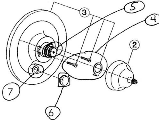
MOUNTING SCREWS+CAM+DIVERTER ASSEMBLY
