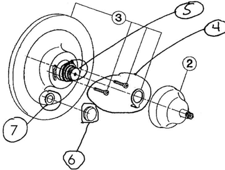
MOUNTING SCREWS+CAM+DIVERTER ASSEMBLY
