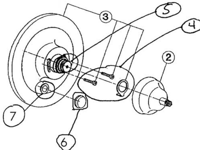
MOUNTING SCREWS+CAM+DIVERTER ASSEMBLY
