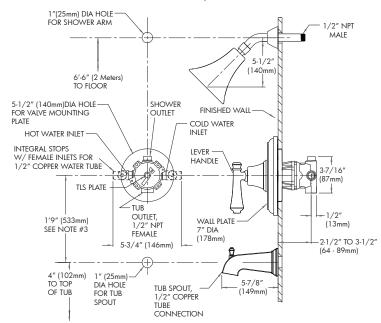
NOTE: 1. All dimensions are in inches (millimeters) unless otherwise specified and are subject to change without notice. 2. Unless otherwise specified, all inlets and outlets are ½" female copper sweat. 3. For ADA mounting locations, consult ADAAG, ANSI A117.1, or static reaulations.
