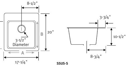
17-1/4" W x 20" D (438 mm x 508 mm) A 14", B 14" Capacity: 7 gallons
