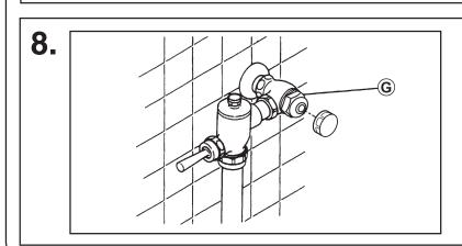
The stop cap screw cover should be replaced and tightly secured after final adjustments have been made.
