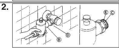
Prior to inserting the flushometer valve tailpiece (B) into the stop valve, be certain that the O-ring seal (C) is located in the O-ring seal groove at the end of the tailpiece, and the locking nut (D) and locking snap ring (E) are located as shown. Care should be taken not to damage the O-ring when inserting the tailpiece into the stop valve. If lubrication is needed, wetting the O-ring with water will be sufficient.
