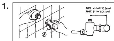
Install stop valve assembly (A) and wall flange. Refer to shown rough in dimension. Thread sealing compounds should be used on male NPT threads only.
