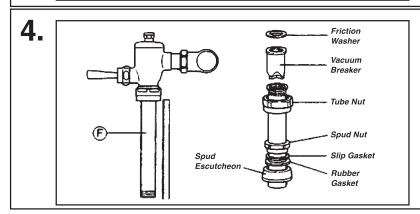
Determine the length of vacuum breaker tube (F) required to join the flushometer valve and fixture spud. Cut the vacuum breaker tube, if required, to this length. Assemble the vacuum breaker tube assembly and spud nut assembly to the flushometer valve and fixture spud.
