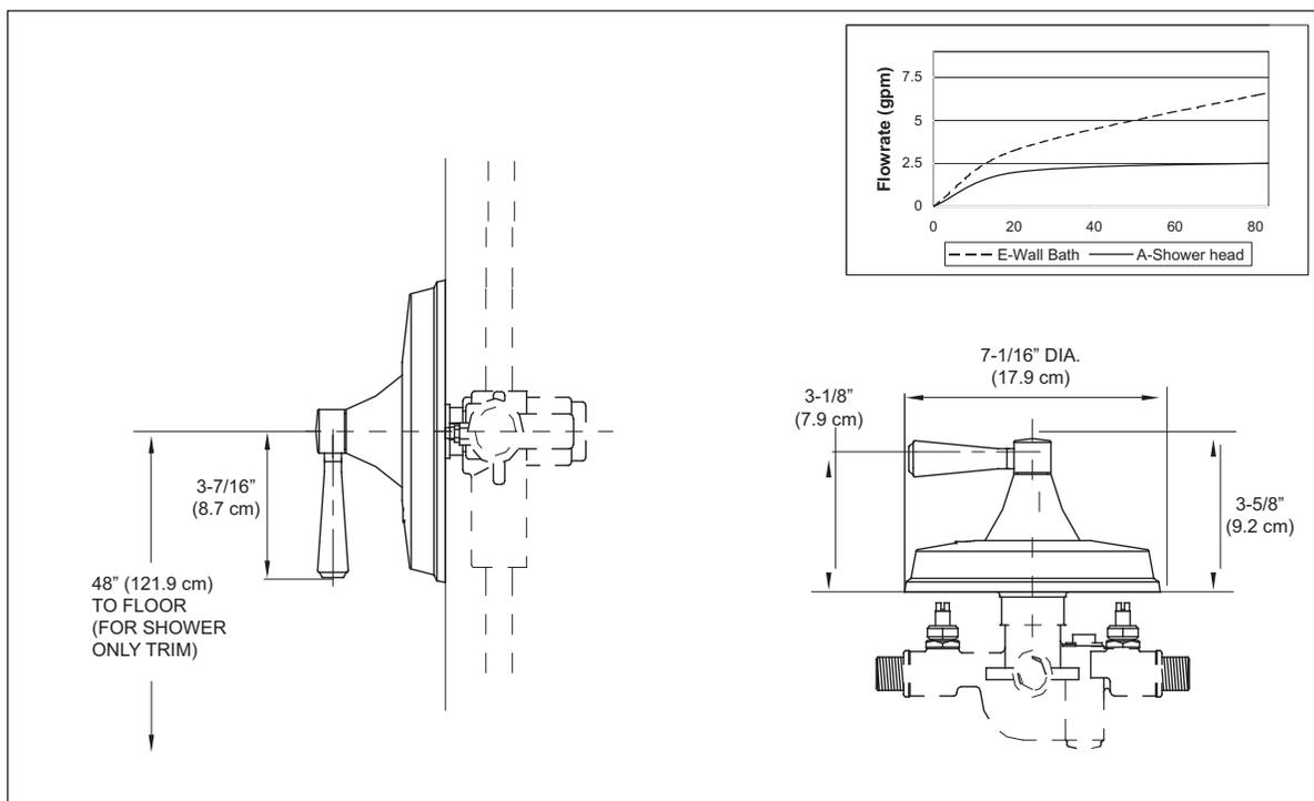
TS784P - Clayton® Pressure Balance Valve Trim without Diverter
