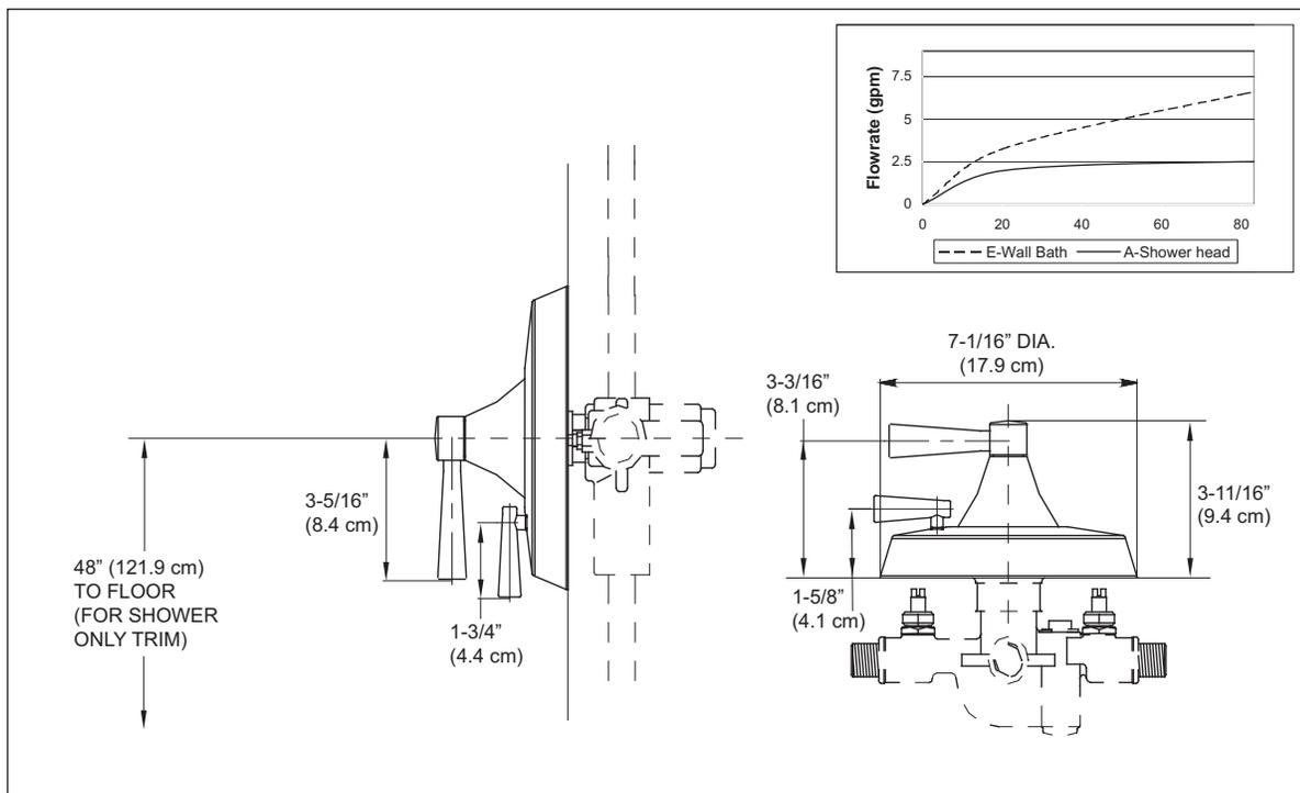
TS794PV - Nexus® Pressure Balance Valve Trim with Diverter
