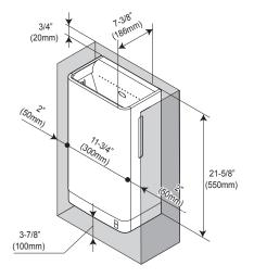
\*\*\*Clearance is required in order to take the water tray, side covers for cleaning and maintenance.
