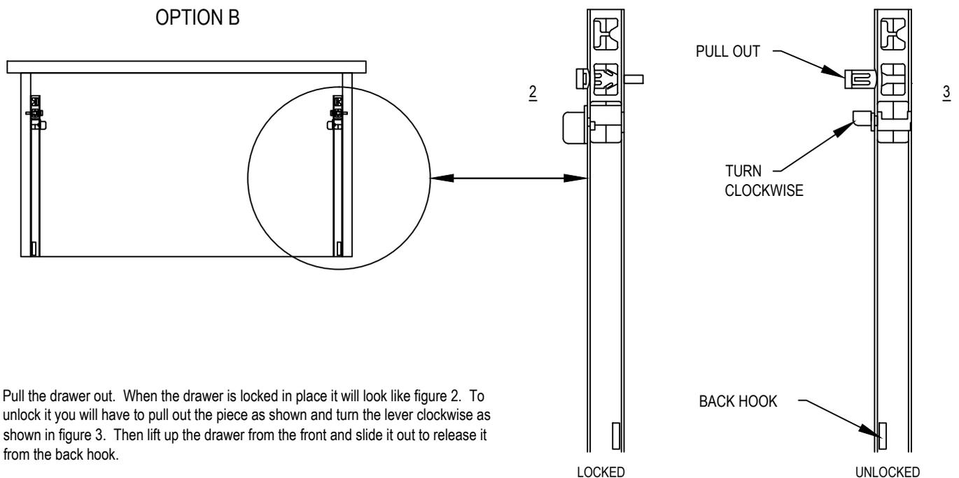
Pull the drawer out. When the drawer is locked in place it will look like figure 2. To unlock it you will have to pull out the piece as shown and turn the lever clockwise as shown in figure 3. Then lift up the drawer from the front and slide it out to release it from the back hook.
