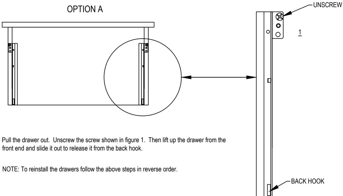
Pull the drawer out. Unscrew the screw shown in figure 1. Then lift up the drawer from the front end and slide it out to release it from the back hook.
