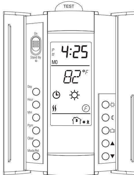
The default Comfort setting is a floor temperature of 82 °F. To modify this temperature, use the **Up** (▲) and **Down** (▼) buttons to reach the desired temperature, and immediately press and hold the **Comfort** (☼) button for 3 seconds. After another 5 seconds, the current floor temperature will again be displayed.
