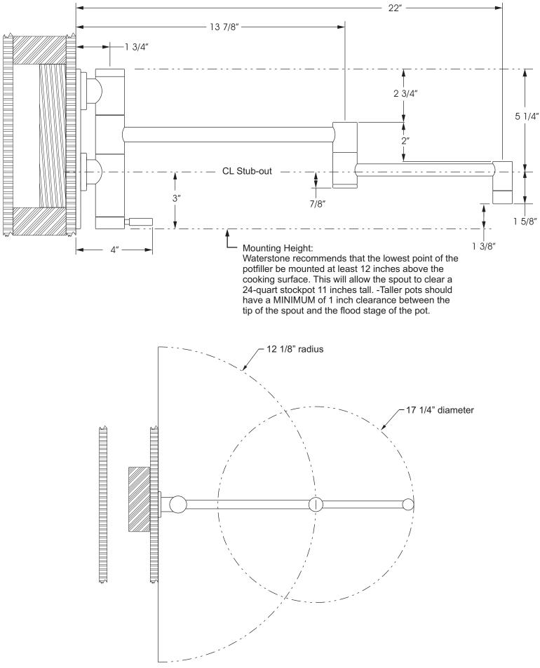
**Maintenance:** Your potfiller is engineered and built with an easily removable aerator in the tip. If the stream of water is not straight and smooth flowing, debris from the household water system may be trapped in the aerator screen. To clean, unscrew the tip and clean any dirt/debris collected on top of the aerator. The tip can be re-installed without any pipe tape or sealant, it has an o-ring seal to make cleaning and re-assembly easy.
