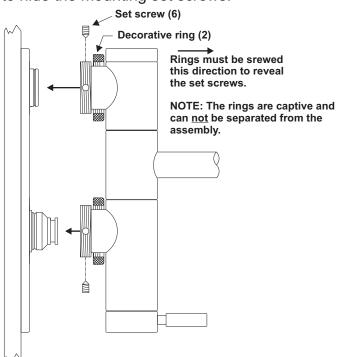
lower three set screws and the upper three set screws using the 3/32" hex wrench provided in your installation kit. DO NOT OVERTIGHTEN THE SET SCREWS. Snug tight and firm is all you need. Once all six set screws are in place, thread the decorative upper and lower rings back onto the mounting bases to conceal the threads and the set screws. Hand tighten only, do not use a wrench.
