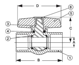
1/2" - 2" VALVES MAX TEMP 113 °F - 230 PSI 2 1/2" - 6" VALVES MAX TEMP 113 °F - 150 PSI
